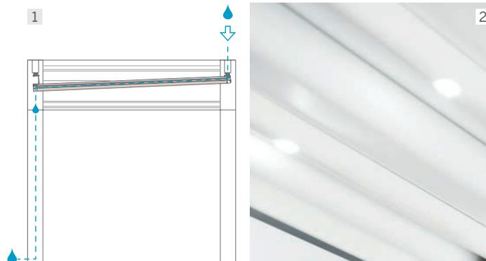
**1. EN lateral drain** The slope of the cloth favors the lateral drainage of water, which flows through the specific pipes inside the frame then onto the ground through the openings at the base of the posts.
