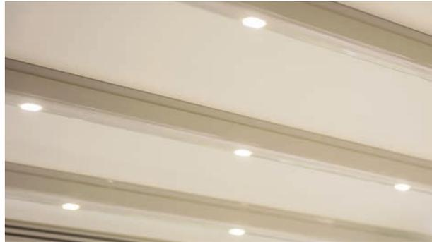
**EN Led Spot integrated in the windbreak bar** (see page 17), with the bar incorporated in the windbreak bar, with groups of 6 leds every 50 cm: **Rectangular led spots** formed of groups of 6 0,5 W leds, for a total of 3 w/spot. Uses around ½ of the light given by the 6 leds. The Led Spotlights can only be installed in the **Plana and Maki cloth systems**.
