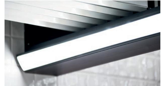
**EN The Raya Led Bar** in aluminum with opal diffuser can be installed on the wall or the internal part of the structure. Neutral light with an adjustable intensity thanks to the dimmer. Color temperature 4000°K, length up to 4 m with 100-Watt power feed, over and up to 6 m with 200-Watt power feed. Standard white paint, other colors upon request. Raya Led Bar can be installed at any moment, regardless of the cloth used.
